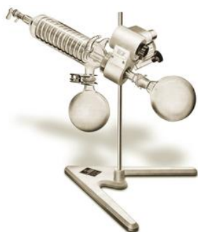
Figure 1: First generation of rotary evaporators with rather flat immersion angles (BUCHI Rotavapor, 1957).
